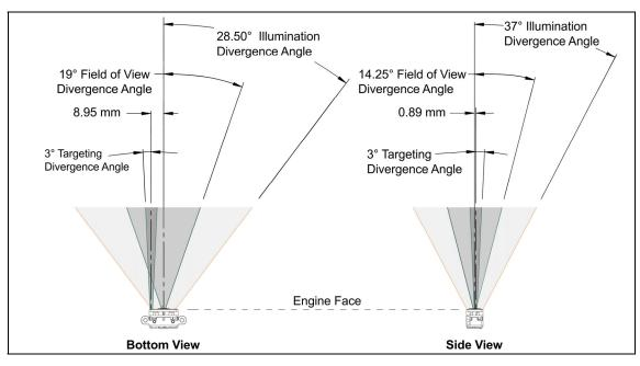
Figure 15. IS4911 Optical Clearance Specifications
